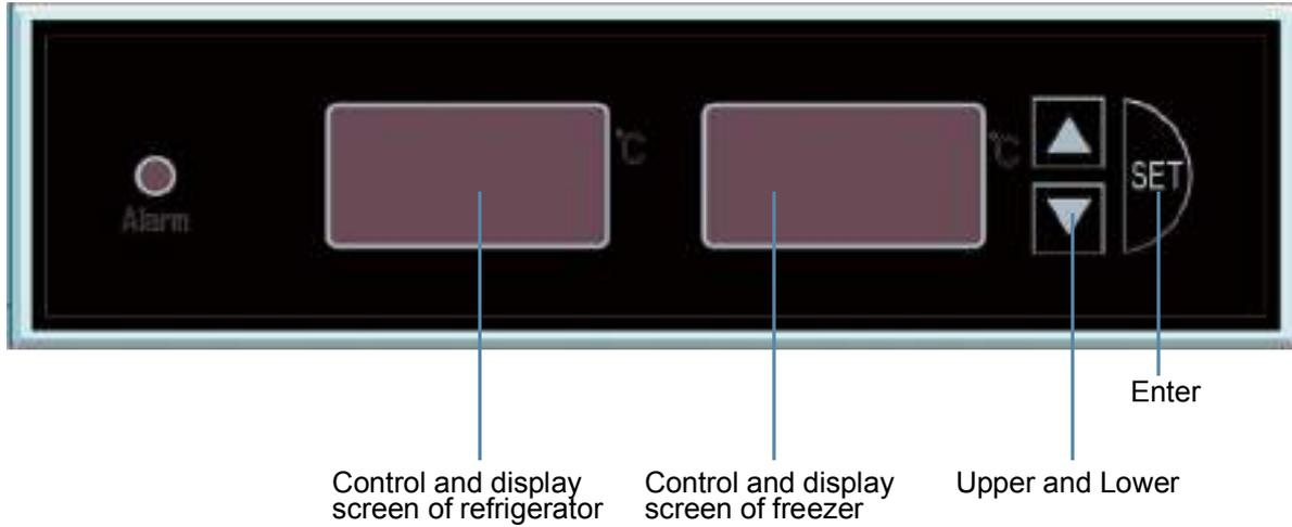
This controller is installed in the electric cabinet for control the work of compressor, fan and heater strip. The parameters have been set before the delivery, which cannot be changed by the user.
