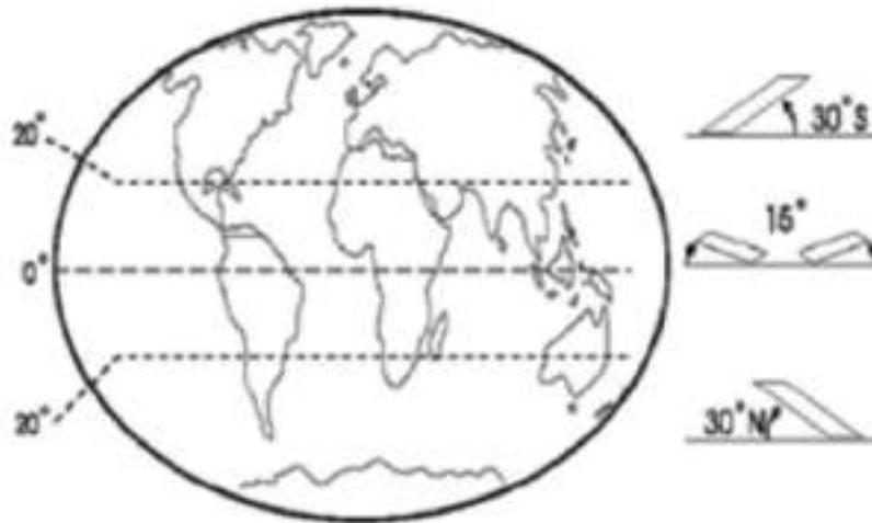
Recommended installation angle of solar panel
